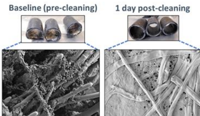
Figure 2. Scanning electron microscopy (SEM) images of the internal feed pipe surface before and after cleaning.
