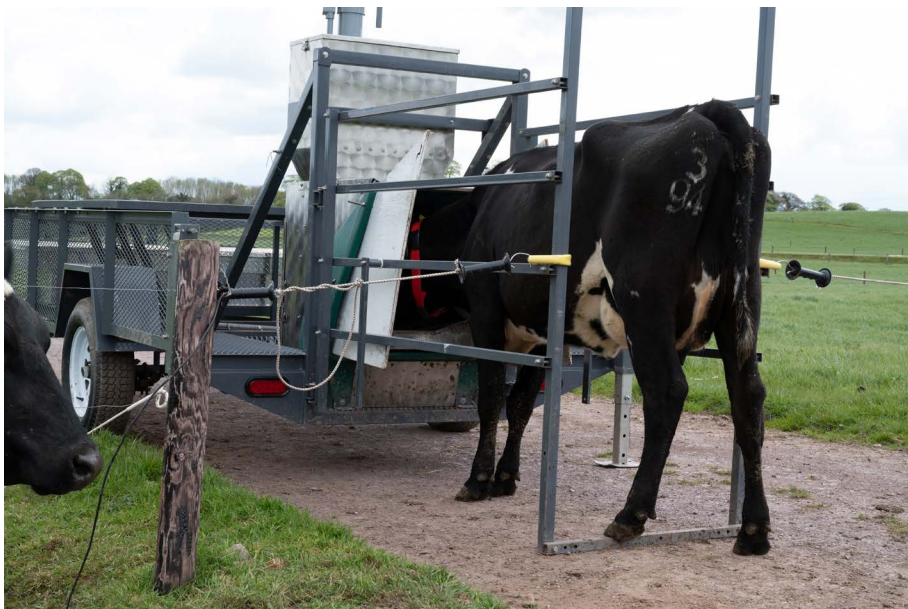
Figure 1. Cow being measured for methane emissions using a GreenFeed unit
