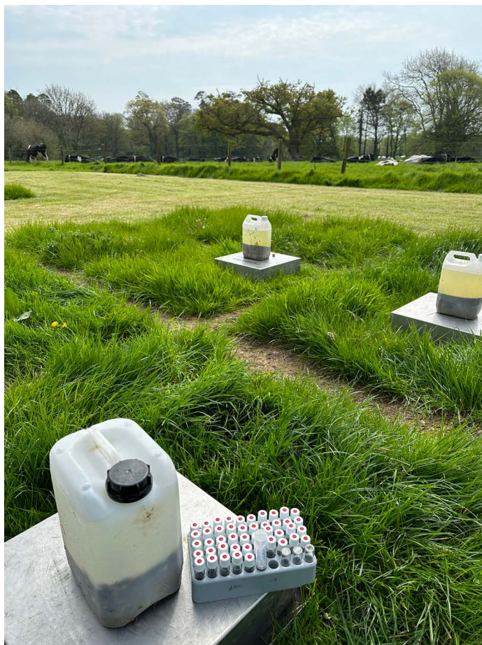
Figure 2. Research quantifying the effect of fertiliser type on nitrous oxide emissions using the closed static chamber technique
