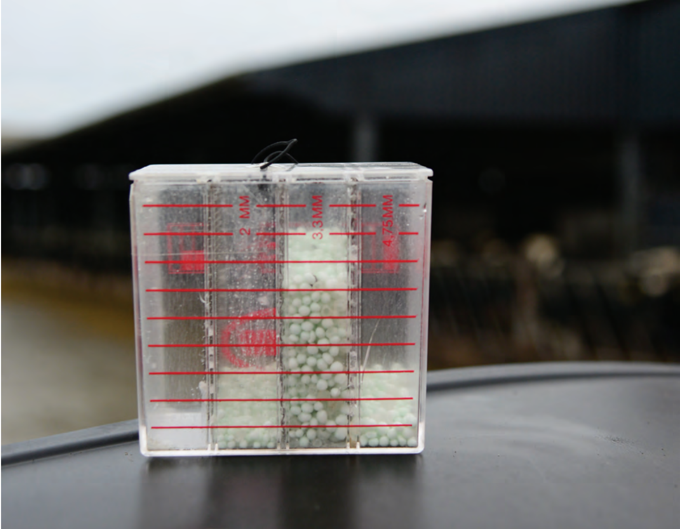
Sieve box: Characterising the fertiliser in terms of granule size distribution, density and strength allows it to be matched to a product in the spreader manufacturers database, giving the correct setting for spreader evenness, which is now normally accessed via a phone app or similar.
