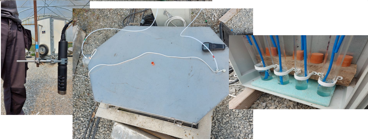
(a) Hanna Multiparameter which is placed into the cattle slurry during treatment in order to measure real-time pH, redox potential, temperature and dissolved oxygen; (b) Mesocosm lid for testing GHG and ammonia; (c) Acid bubblers for scrubbing ammonia from sampled air for further analyses during dynamic chamber testing
